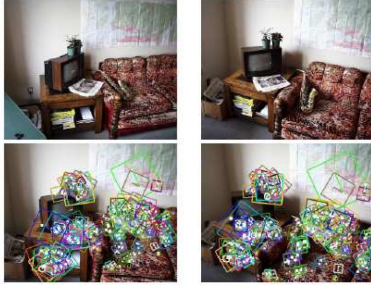
Figure 4.2: Matching using color descriptors over color images done by Fergus et al.
