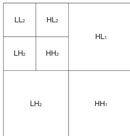
Figure 2.5: 2 Scale 2-Dimensional Discrete Wavelet Transform
