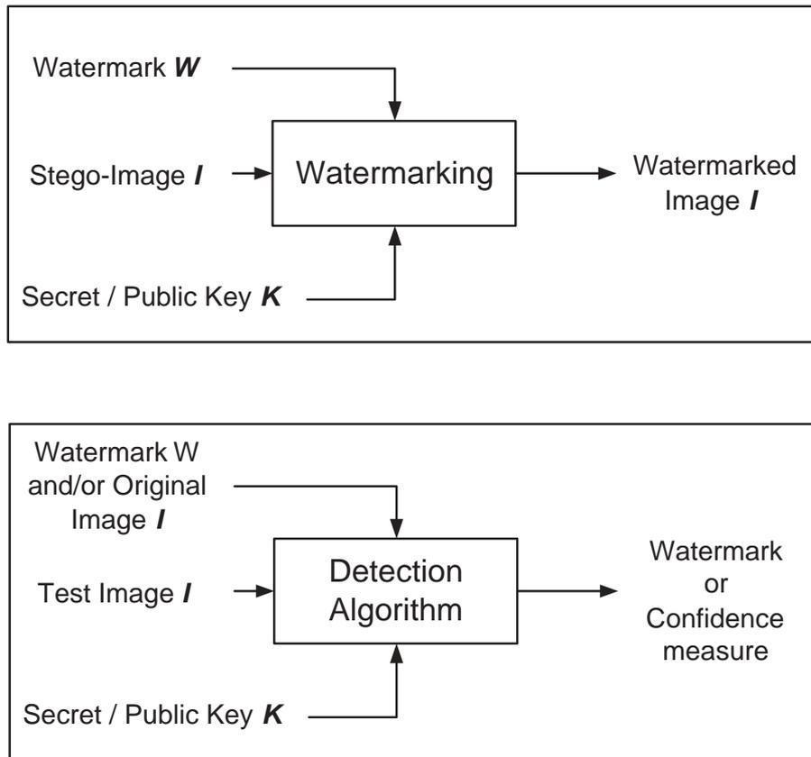
Figure 2.3: Watermarking Embedding and Detection Scenario
