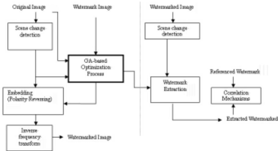
Figure 3.22: The GA-based watermarking algorithm
