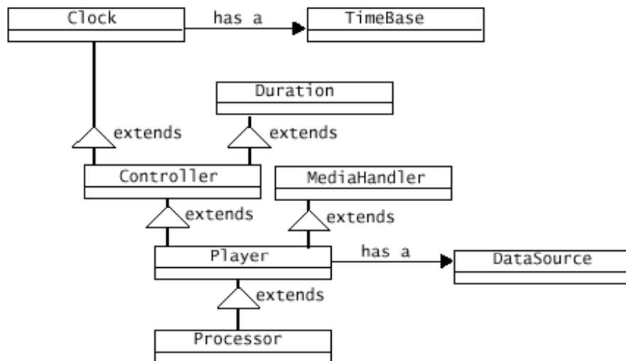
In JMF, the presentation process is modeled by the Controller interface. Controller defines the basic state and control mechanism for controls, presents, or captures time-based media. It defines the phases that a media controller goes through and provides a mechanism for controlling the transitions between those phases. A number of the operations that must be performed before media data can be presented can be time consuming, so JMF allows programmatic control over when they occur.
