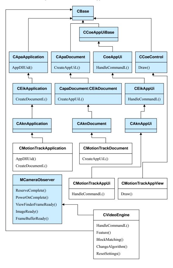
This diagram shows the classes implemented by MotionTrack application, and which files implement those classes. All the classes are derived from CBase. CBase has a number of useful features: it initialises all member data to zero, it has a virtual destructor, and it implements support for the Symbian OS cleanup stack.
