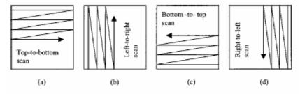
Fig. 1 Various matching scans: (a) Top-to-bottom scan, (b) left-toright scan, (c) bottom-to-top scan, (d) right-to-left scan.
