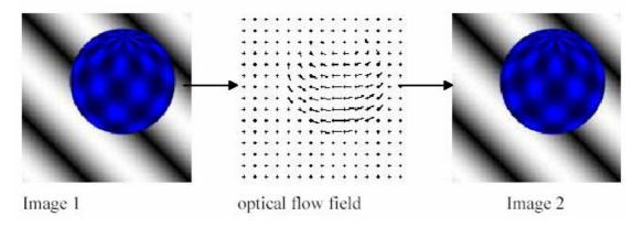
Figure 5.13 Illustration of Optical Flow
