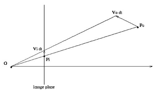
Figure 5.14 Object motion creates a motion field on the 2D image plane
