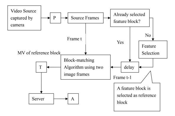
Figure 7.1 Flow Chart of developing motion tracking application
