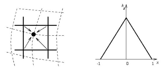
Figure 26: Linear interpolation and its brightness function.
