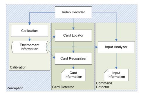
Figure 6: the architecture of Perception Module
