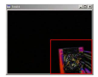
Figure 13: Resulting image of comparing current frame and previous frame.
