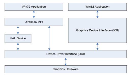
Figure 9: the system integration of Direct3D
