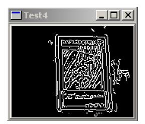
Figure 18: Resulting image after applying Canny algorithm.
