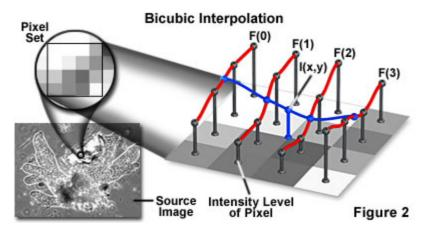
Figure 27: Illustration of bicubic interpolation.
