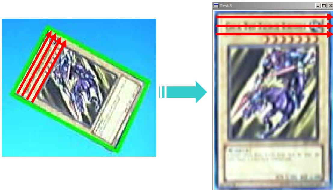
Figure 24: The distorted card image (left) and the resulting undistorted card image (right).
