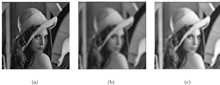
Fig. 3. The Example of blind image restoration by IPEM. (a) The original Lenna image, (b) The blurred image, (c) The restored image
