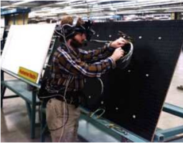
Figure 10. A researcher demonstrates Boeing's prototype wire bundle assembly application. (Courtesy David Mizell, Boeing)[9]
