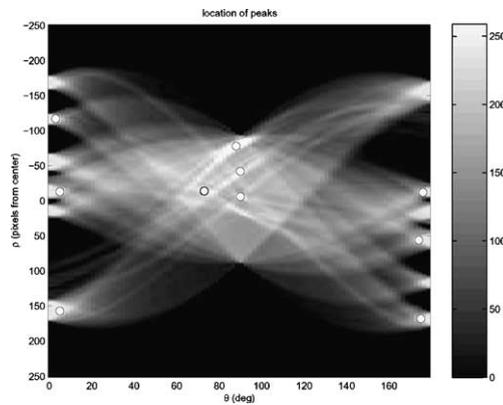
Fig. 11. “Peaks” of Hough transform without edge detection.
