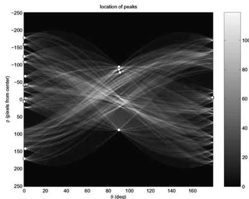
Fig. 12. “Peaks” of Hough transform after edge detection.
