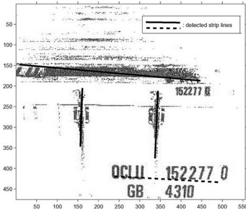
Fig. 23. Four detected strip lines.
