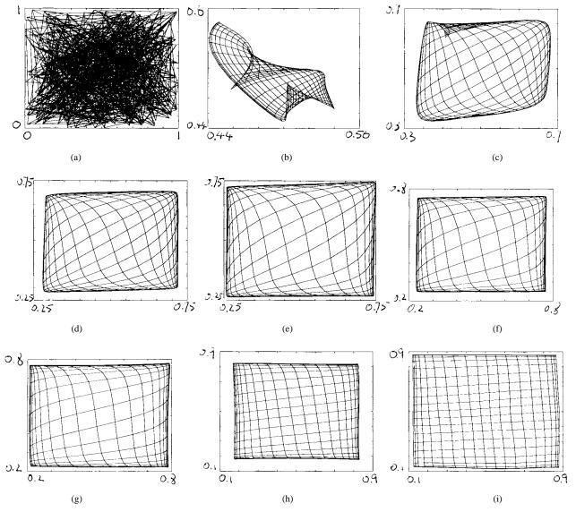
Fig. 2 The topographic map formation in the simulation of  $15 \times 15$  map at the time when (a) t = 0, (b)  $t = 10^6$ , (c)  $t = 2 \times 10^6$ , (d)  $t = 3 \times 10^6$ , (e)  $t = 4 \times 10^6$ , (f)  $t = 5 \times 10^6$ , (g)  $t = 6 \times 10^6$ , (h)  $t = 7 \times 10^6$ , and (i)  $t = 8 \times 10^6$ .
