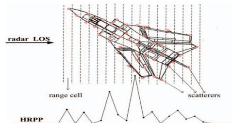
**Fig. 1.** Radar returns from the scatterers on the target are projected onto the LOS, resulting in an HRRP.
