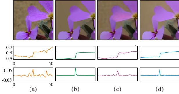
Figure 1. Learning operations using color- and gradient-domain constraints. (a) Input image. (b)  $L_0$  smoothing effect to learn. (c) Learning result on image color. (d) Learning result on image gradient.
