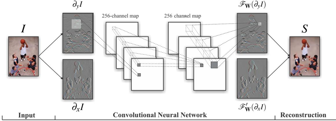
Figure 2. A unified learning pipeline for various edge-aware filtering techniques. The main building blocks are a 3-layer deep convolutional neural network and an optimized image reconstruction process.
