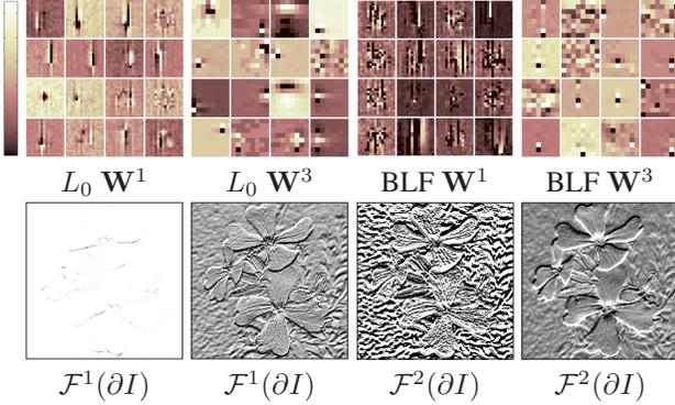
Figure 3. Visualization of intermediate results from hidden layers. The top row shows the selected weights trained for  $L_0$  smoothing and bilateral filter. The bottom row shows the hidden layer activation for the bilateral filter.
