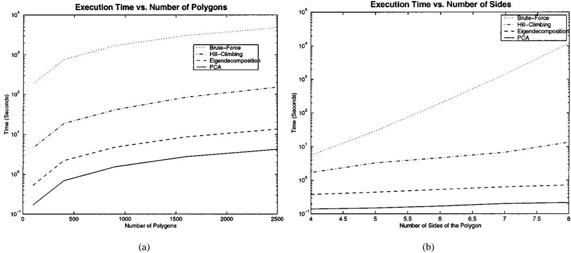
Fig. 3. (a) Execution time versus number of polygons plot illustrates the computational time required for each of the four algorithms to perform for various polygons with six sides. (b) Execution time versus number of sides plot illustrates the computational time required for each of the four algorithms to perform for various sides of 100 polygons.
