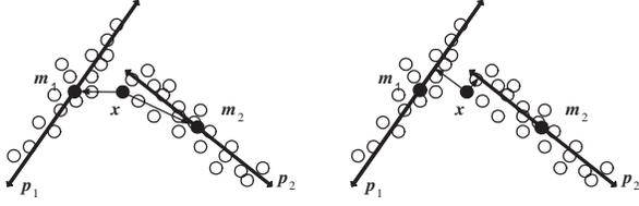
Figure 1: Assignment of the data point  $\vec{x}$  to one of two regions based on (left) Euclidean distance, and (right) the reconstruction distance. The mean  $\vec{m}_i$  and leading eigenvector  $\vec{v}_i$  are shown for each of two regions ( $i = 1, 2$ ).
