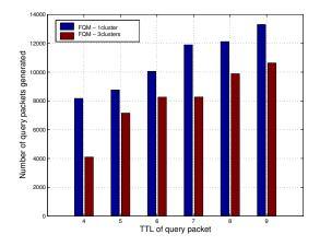
Figure 4.19: Generated Network Traffic against TTL value of query packet
