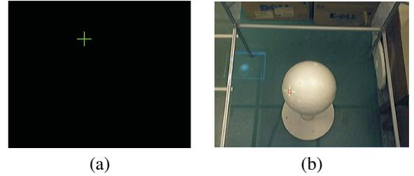
Fig. 4. Finding correspondence between the projector and camera image. (a) The cross image projected to the sphere; (b) The cross image observed by the camera.
