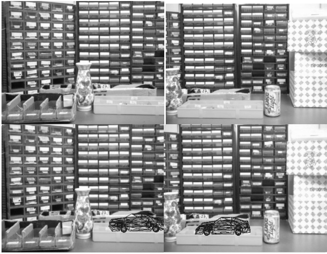
Fig. 6. Results of inserting an artificial object into the test scene using our IMM-based approach. First row: The first and the last image of the test sequence. Second row: A synthetic car, which was drawn by wire-frames, was put into the real scene. More results can be found at http://www.cse.cuhk.edu.hk/~khwong/demo/
