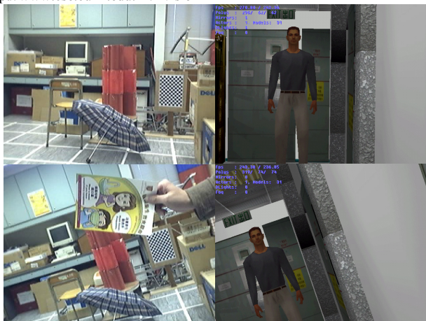
Fig. 4. Application of the motion recovered from the hand-held sequence to virtual reality. The 1 st row shows the right view of the original (left) and resulting virtual (right) stereo sequence. The 2 nd row illustrates the right view of the 77 th image pair of the real (left) and virtual reality (right) sequence.
