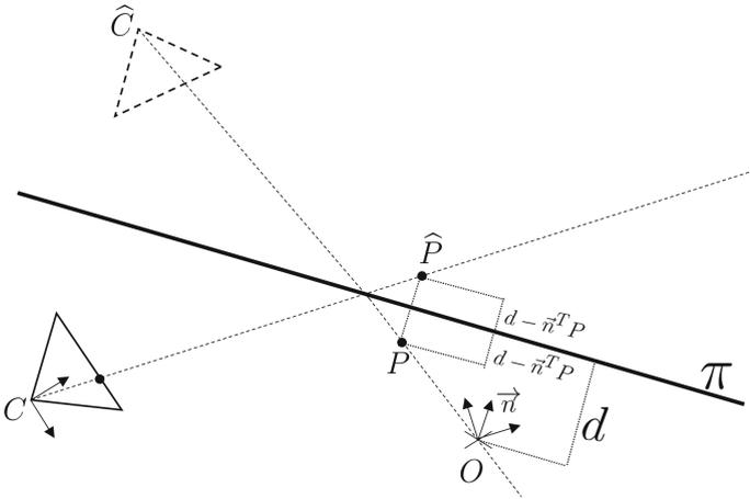
**Fig. 2.** Overview of mirror geometry.  $P$  is a 3-D point and  $\hat{P}$  is its reflection.
