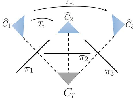
**Fig. 3.** Mirrors  $\pi_i$  and virtual cameras  $\hat{C}_i$
