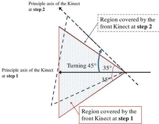
Fig. 5. The region captured by the front Kinect at step 1 and step 2
