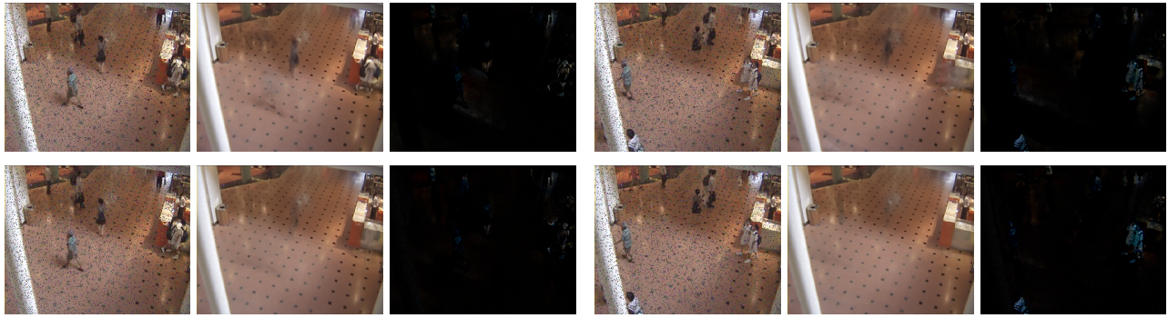
Figure 6: Foreground and background separation results of different algorithms on the Mall data set, where the first and second rows show the recovered low-rank and sparse images by GRASTA and RMCMF, respectively.
