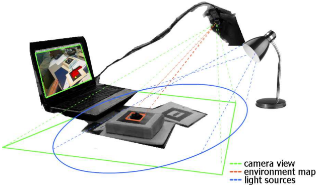
Fig. 1. The setup used for estimating light source position using a laptop computer and a standard consumer web-camera
