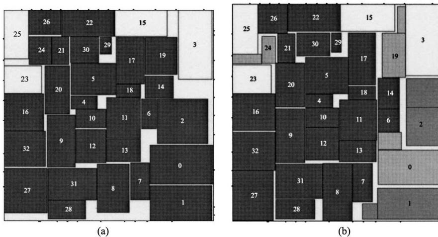
Fig. 8. Data set ami33 with hard modules and boundary constraints. (a) Preliminary floorplan. Deadspace = 8.99%. Module 3, 15, 23 and 25 are hard blocks with boundary constraint. (b) After sizing and shaping. Deadspace = 5.77%.
