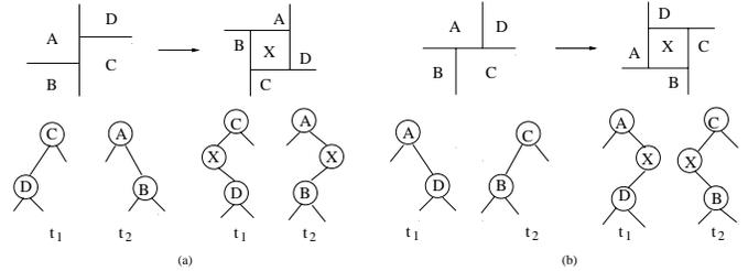
Figure 9: Mapping between mosaic floorplan and non-slicing floorplan
