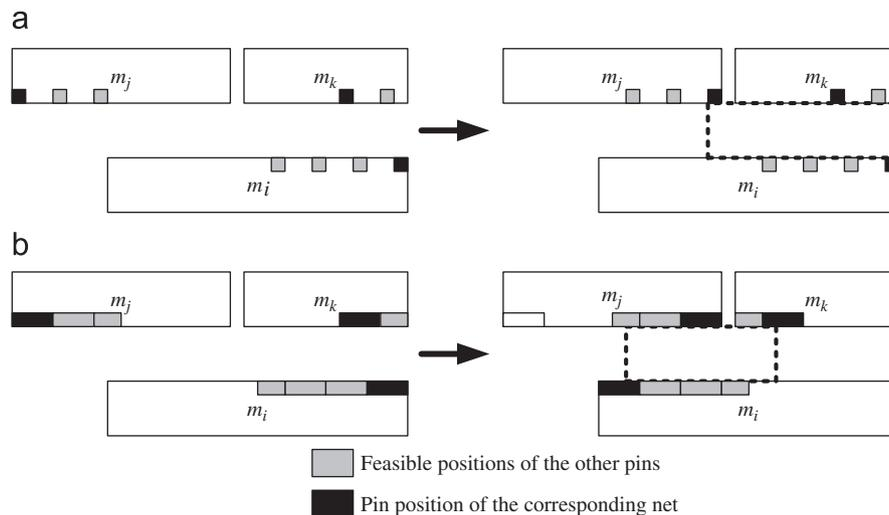
Fig. 1. Example of block flipping with floating pins.
