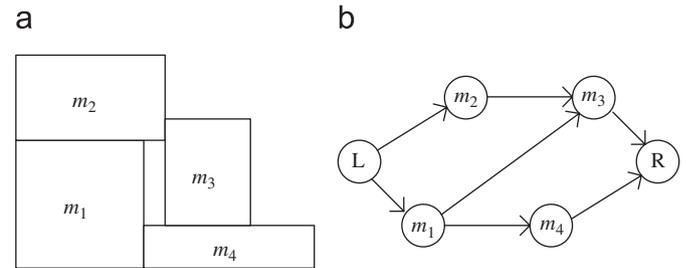
Fig. 7. Example of constructing a constraint graph for a floorplan. (a) Floorplan; (b) horizontal constraint graph.
