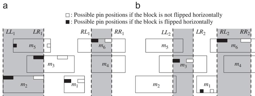
Fig. 4. An example of independent block: (a) a net  $n_1$  connecting to  $m_1, m_2, m_3, m_5$  and  $m_6$  and (b) a net  $n_2$  connecting to  $m_1, m_3$  and  $m_6$ .
