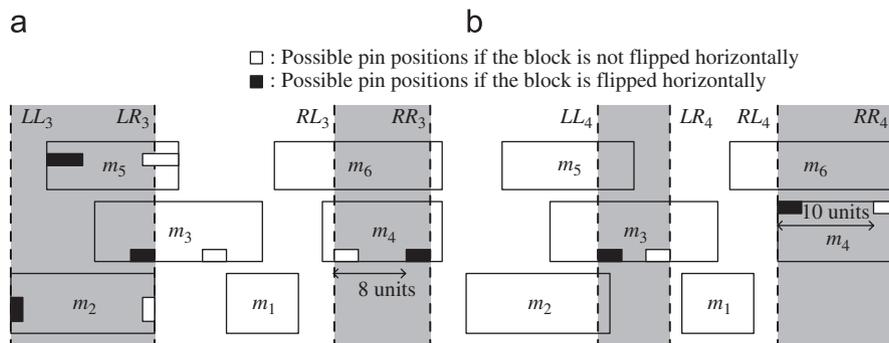
Fig. 5. An example of strictly solvable block: (a) a net  $n_3$  connecting to  $m_2, m_3, m_4$  and  $m_5$  and (b) a net  $n_4$  connecting to  $m_3$  and  $m_4$ .
