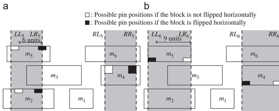
Fig. 6. An example of conditionally solvable block  $m_5$ : (a) a net  $n_5$  connecting to  $m_2$ ,  $m_4$  and  $m_5$  and (b) a net  $n_6$  connecting to  $m_4$  and  $m_5$ .
