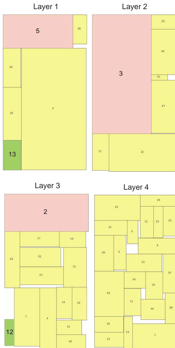
Figure 6: A result packing of ami49 in Data set 3 ( B_1 = \{0-5, 32, 33, 44\} , B_2 = \{6-11\} , B_3 = \{12-17\} ).
