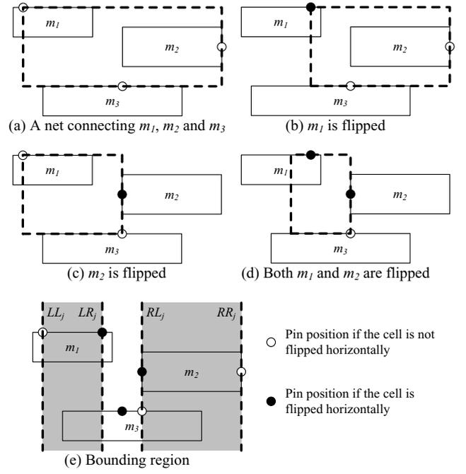
Figure 1: An Example of Bounding Box and Bounding Region of a Net  $n_j$
