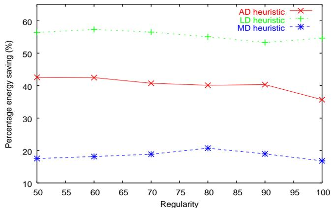
Fig. 9. Percentage energy saving as a function of regularity for MD, AD and LD heuristics.
