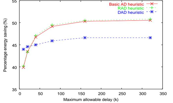
Fig. 5. Percentage energy saving as a function of  $k$  for AD, RAD and DAD heuristics.
