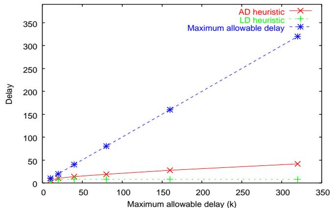
Fig. 11. Maximum allowable delay as compared to the actual observed delay for AD and LD heuristics.
