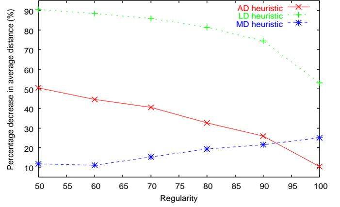
Fig. 8. Percentage decrease in average distance as a function of regularity for MD, AD and LD heuristics.
