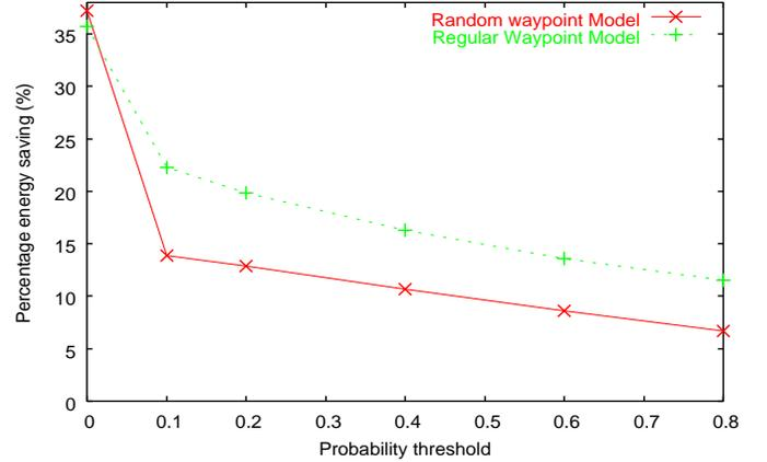
Fig. 1. Percentage energy saving as a function of  $p_{th}$  for MD heuristic.
