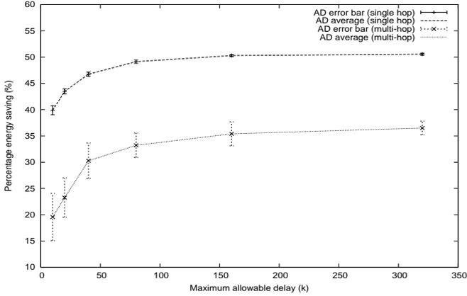
Fig. 3. Percentage energy saving as a function of  $k$  for AD heuristic.
