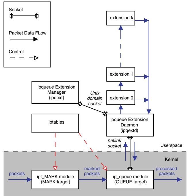
Fig. 3. Overview of the user-space extension architecture.
