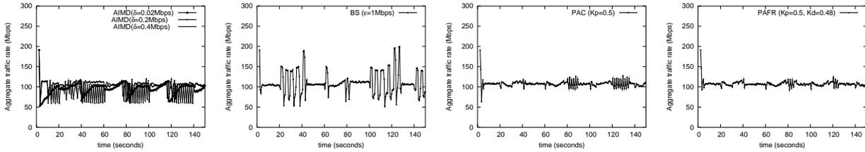
Fig. 8. (a) AIMD algorithm with step size of  $\delta = 0.02M$  ( $T_s = 9.3s, J = 114Mb$ ),  $\delta = 0.2M$  ( $T_s = 2.0s, J = 28.1Mb$ ) and  $\delta = 0.4M$  ( $T_s = 16.1s, J = 236.4Mb$ ). (b) Binary Search algorithm.  $\epsilon = 1M$  ( $T_s = 9.8s, J = 229.2Mb$ ). (c) PAC ( $K_P = 1/2$ ) algorithm ( $T_s = 2.4s, J = 12.9Mb$ ). (d) PAFR algorithm with  $K_P = 0.5$  and  $K_D = 0.48$  ( $T_s = 1.3s, J = 7.1Mb$ ).
