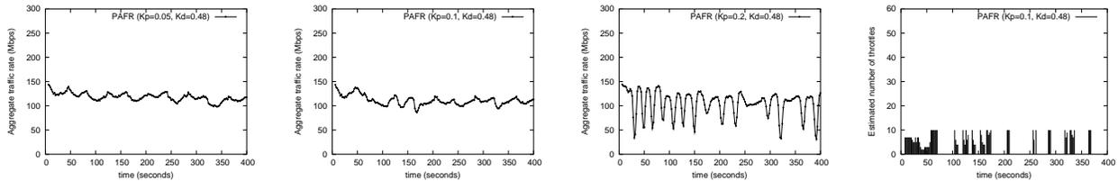
Fig. 14. Performance of the PAFR throttle algorithm with complete information that  $|R(k)|_{\max} = 10$ ,  $K_D = 0.48$  as  $K_P$  takes the value of (a)  $K_P = 0.05$  ( $T_s = 35.4s$ ,  $J = 286.8Mb$ ), (b)  $K_P = 0.1$  ( $T_s = 19.5s$ ,  $J = 145.0Mb$ ) and (c)  $K_P = 0.2$  ( $T_s = 60.0s$ ,  $J = 790.1$ ). (d) Estimated number of effective throttles using the  $est()$  algorithm for the case  $K_P = 0.1$ .
