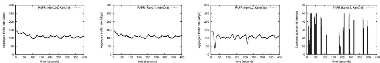
Fig. 13. Performance of the PAFR throttle algorithm with an estimate that  $|R(k)|_{\max} = 50$ ,  $K_D = 0.48$  as  $K_P$  takes the value of (a)  $K_P = 0.05$  ( $T_s = 13.4s$ ,  $J = 92.0Mb$ ), (b)  $K_P = 0.1$  ( $T_s = 8.6s$ ,  $J = 50.6Mb$ ) and (c)  $K_P = 0.2$  ( $T_s = 13.5s$ ,  $J = 71.0Mb$ ). (d) Estimated number of effective throttles using the  $est()$  algorithm for the case  $K_P = 0.1$ .
