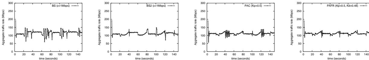
Fig. 12. (a) Binary Search (BS) with  $\epsilon = 1M$  ( $T_s = 3.9$ ,  $J = 47.0Mb$ ). (b) Improved binary search with  $\epsilon = 1M$  ( $T_s = 1.5s$ ,  $J = 12.9Mb$ ). (c) PAC algorithm with  $K_p = 1/2$  ( $T_s = 3.2$ ,  $J = 19.4Mb$ ) (d) PAFR algorithm with  $K_p = 0.5$ ,  $K_D = 0.48$  ( $T_s = 1.0s$ ,  $J = 7.2Mb$ ). As compared to EXP B, a larger  $[L_s, U_s]$  reduces the cost  $J$ .
