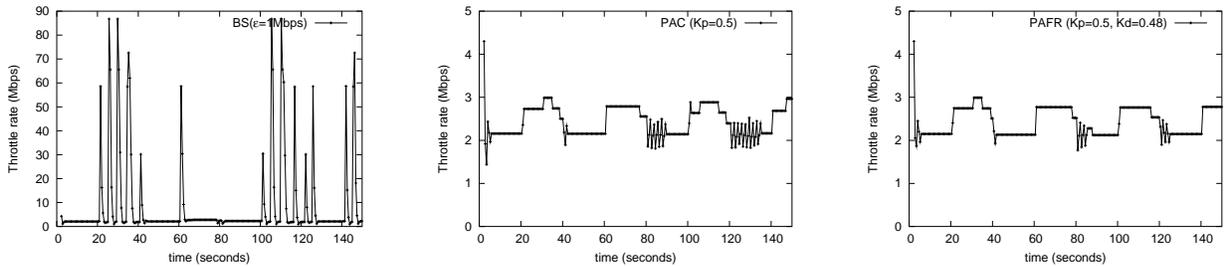
Fig. 9. (a) Binary Search algorithm exhibits large rate throttle variation. (b) PAC ( $K_P = 0.5$ ) algorithm. Significantly large rate throttle variation is observed in the transient response. (c) PAFR algorithm with  $K_P = 0.5$  and  $K_D = 0.48$ . Damping provides better transient response while maintaining excellent response time.
