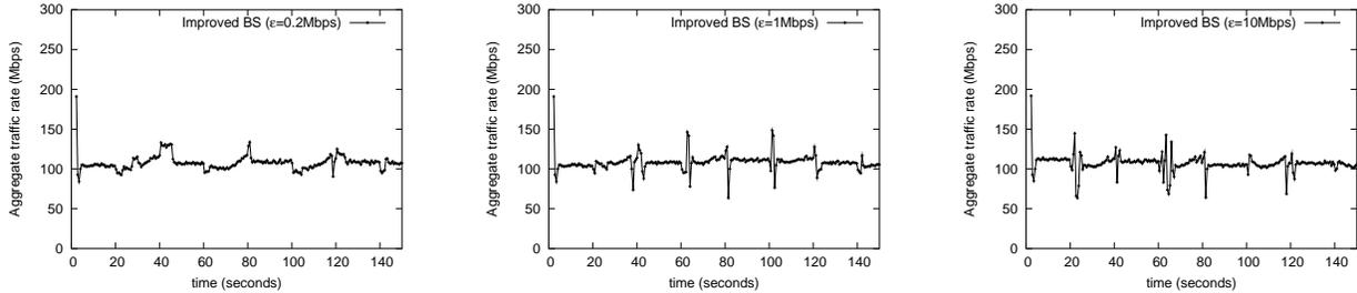
Fig. 11. Improved Binary Search (BS) algorithm with (a)  $\epsilon = 0.2M$  ( $T_s = 3.7s$ ,  $J = 27.0Mb$ ), (b)  $\epsilon = 1M$  ( $T_s = 1.7s$ ,  $J = 13.2Mb$ ), and (c)  $\epsilon = 10M$  ( $T_s = 2.3s$ ,  $J = 28.7Mb$ ).
