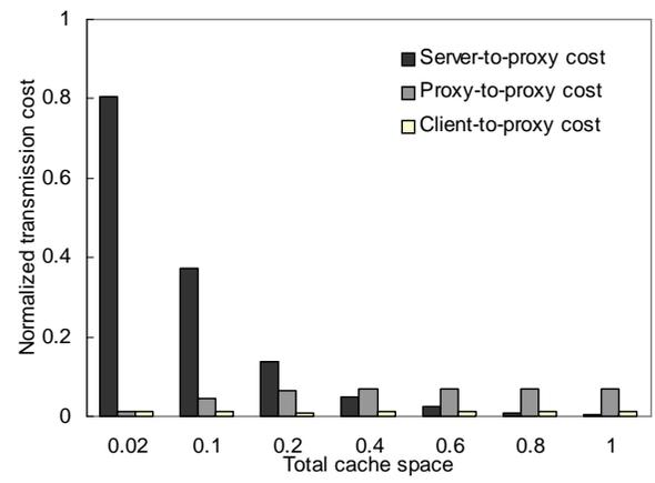
Fig. 5. Transmission cost as a function of the total proxy-client cache space.  $S^p : S^c = 1 : 1$
