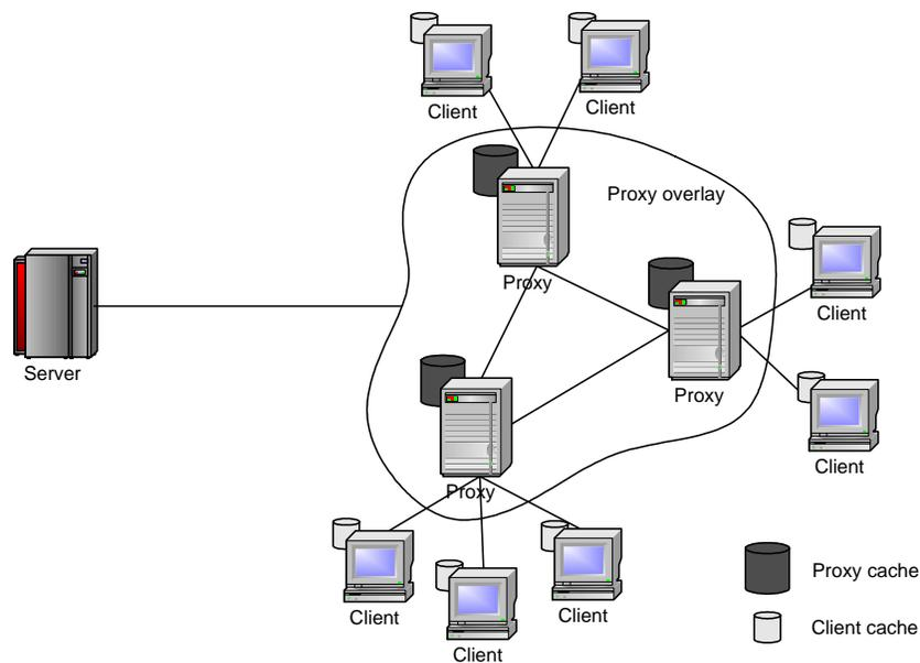
Fig. 1. The cooperative proxy-client caching architecture.
