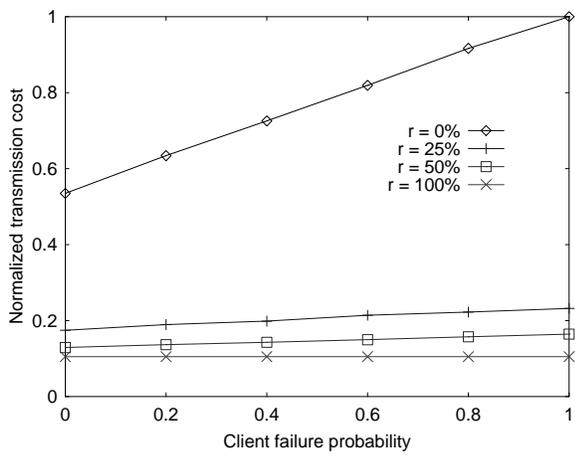
Fig. 9. Transmission cost versus client failure probability.
