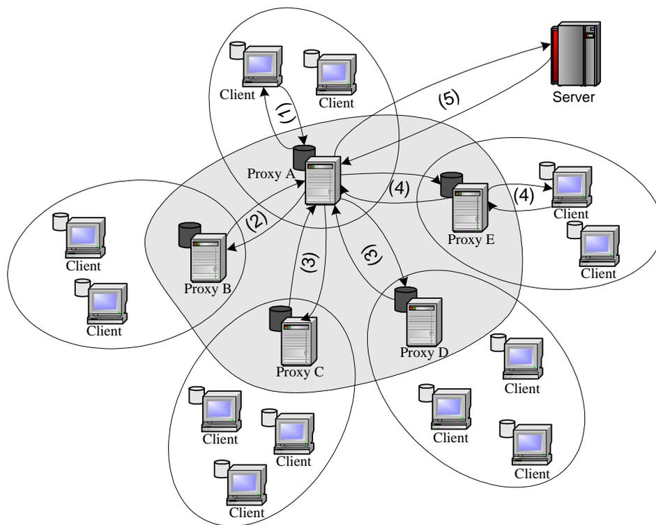
Fig. 4. An illustration of the cache lookup and retrieval operations. (1) client request to home proxy for video  $i$ ; (2) location lookup request to proxy  $B = h(i)$ ; (3) retrieve and relay prefix segments from proxy cache; (4) retrieve and relay prefix-of-suffix segments from clients; (5) retrieve and relay the remaining part of suffix from server.
