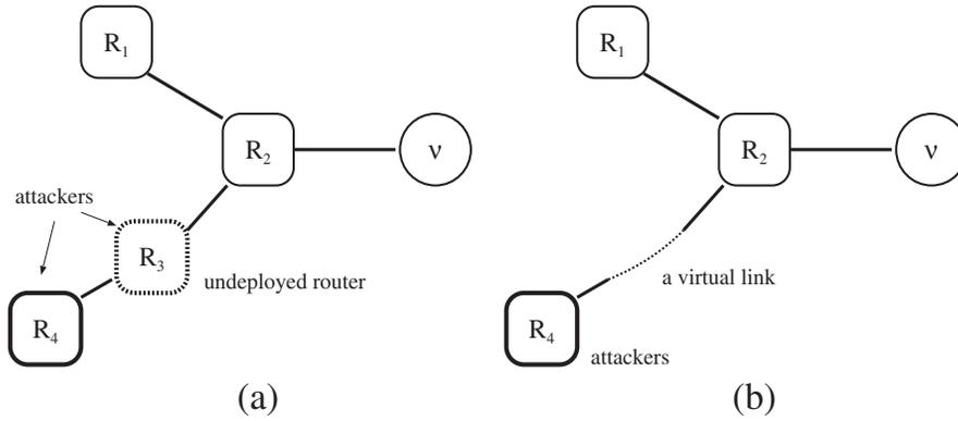
**FIGURE 17.** (a) The same network example as Figure 6 with attacking domains  $R_3$  and  $R_4$ . But the router  $R_3$  is an undeployed router. (b) Logically, a virtual link between the router  $R_2$  and  $R_4$  is formed.
