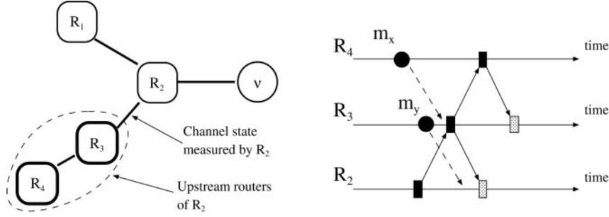
**FIGURE 9.** The channel state of  $Link_{32}$  contains pre-monitoring (monitoring) packets from both  $R_3$  and  $R_4$  in the first (second) instance of the snapshot algorithm.
