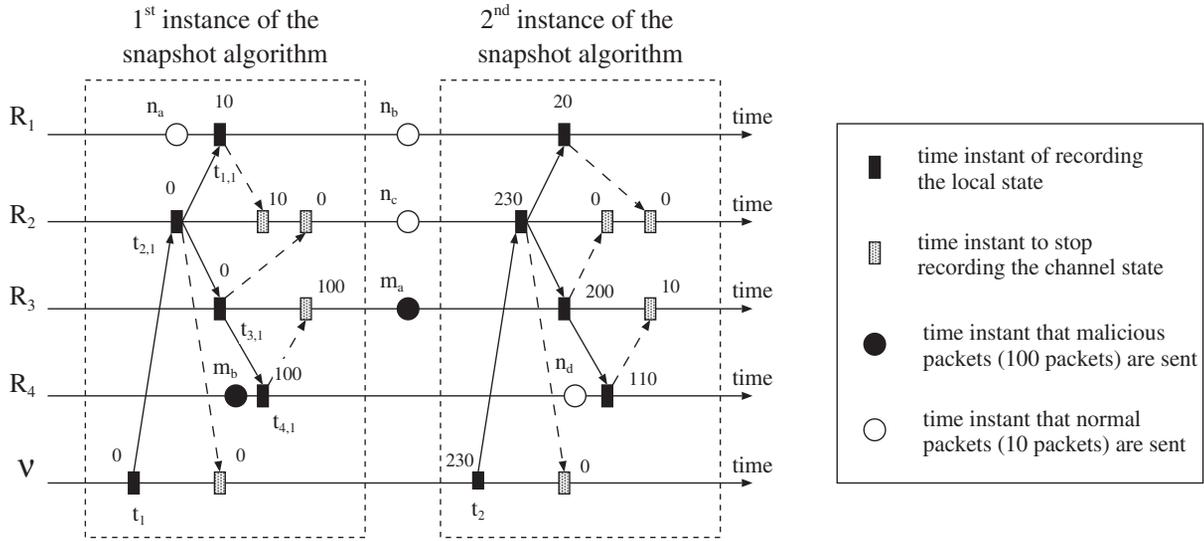
FIGURE 7. A timing diagram that shows the progress of the DDoS traceback algorithm.
