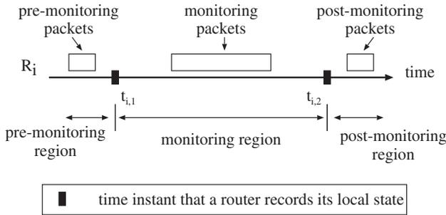
**FIGURE 8.** Classification of pre-monitoring, monitoring and post-monitoring packets.
