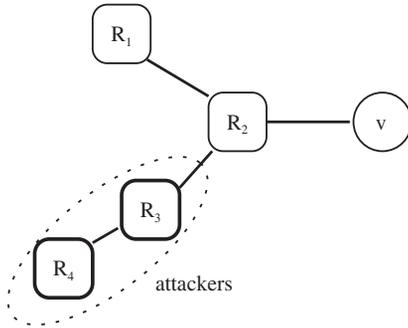
**FIGURE 6.** A network topology with two attackers who reside in the local domains of  $R_3$  and  $R_4$ .
