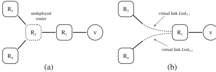
**FIGURE 19.** (a) In this example network, the router  $R_2$  is an undeployed routers while the others are deployed routers. (b) As the undeployed router is transparent to the traceback protocol, the router  $R_1$  records the channel state of the virtual links  $Link_{3,1}$  and  $Link_{4,1}$ .
