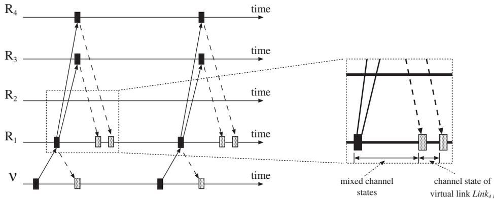
**FIGURE 20.** The timing diagram under a partial deployment environment. A drawback is that the channel states of the virtual links  $Link_{3,1}$  and  $Link_{4,1}$  become indistinguishable at router  $R_1$ .
