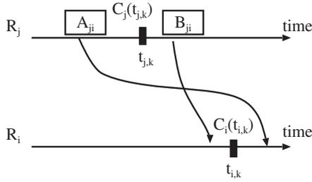
**FIGURE 3.** Correct accumulative local traffic without clock synchronization.
