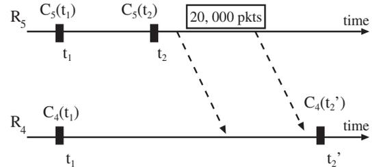
**FIGURE 2.** Asynchronous reading of outgoing traffic counters in Example B.
