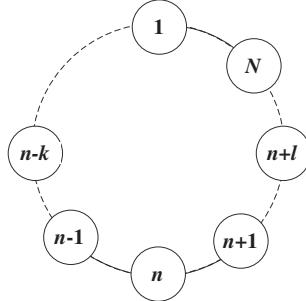
Fig. 3.2. Ring topology with  $N$  nodes.
