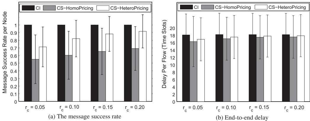
**Fig. 6.10.** Dynamics of system performance vs. the injected credit ratio. The bars in (a) show the average per node message success rate over  $10^6$  runs. The bars in (b) show the average per flow delay over  $10^6$  runs. Standard deviations are shown using lines.
