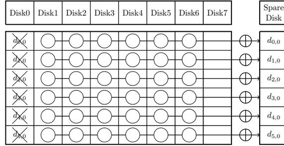
Fig. 4. Conventional scheme to recover Disk 0 of RDP code.
