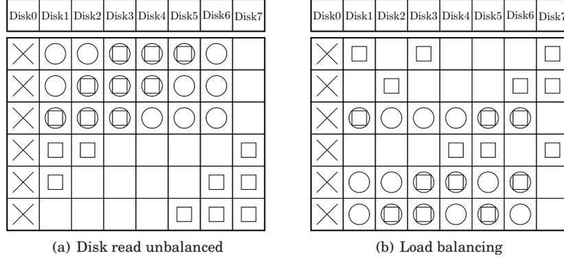
Fig. 5. (a) Reducing the number of disk reads for recovering Disk 0 of RDP code. (b) Load balancing in recovering Disk 0.
