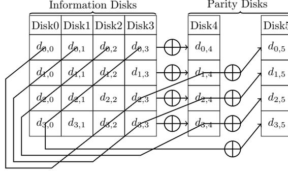
Fig. 2. RDP coding in a stripe of  $p = 5$ .
