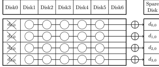
Fig. 7. Conventional scheme to recover Disk 0 of EVENODD code.
