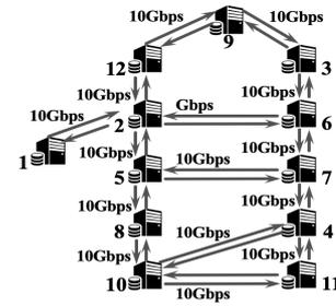
Fig. 4. Topology of the Abilene network.
