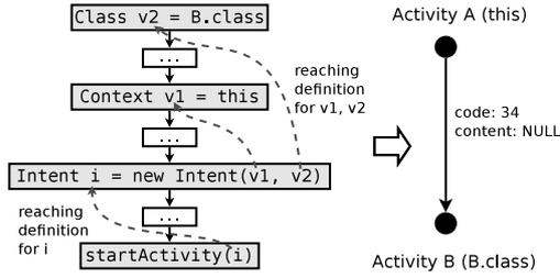
Fig. 4. Data-flow analysis for generating the static behavior graph (SBG).
