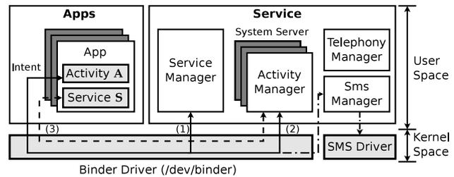
Fig. 1. Intent and binder mechanism.
