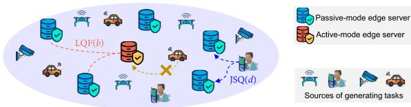
Fig. 1. An illustrative scenario with  $M = 10$  sources,  $N = 5$  passive-mode edge servers, and  $K = 1$  active-mode edge server. The edge servers can be interconnected via a metropolitan-area-network or local-area-network.
