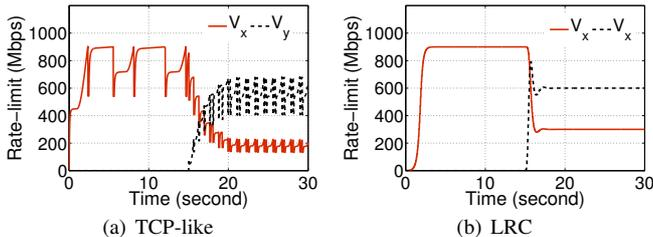
Fig. 9. Rate-limit of VMs with  $w_X : w_Y = 1 : 2$  and no guarantees. ( $v_X$  and  $v_Y$  are the calculated rate-limits of the algorithms)
