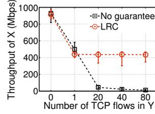
Fig. 6. Throughput of  $X$  (450Mbps guarantee) with different number of TCP flows of  $Y$ .
