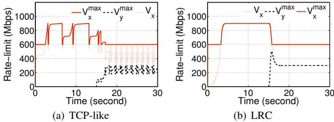
Fig. 8. Rate-limit of VMs with  $B_X = 600\text{Mbps}$ ,  $B_Y = 0$  and the same weight. ( $v_X^{\max} = \max\{v_X, B_X\}$  and  $v_X$  is the rate-limit of the algorithms)
