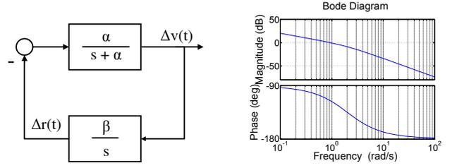
(a) Block diagram of closed loop. (b) Bode diagram ( $\alpha = 2, \beta = 1$ ).
