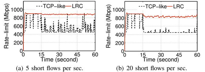
Fig. 10. Rate-limit of  $X$  (450Mbps guarantee) with arrival of short flows at 15<sup>th</sup>s: 5 flows/s at average 17.4Mbps and 20 flows/s at average 66.2Mbps.
