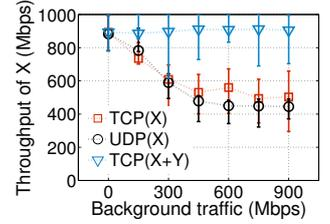
Fig. 7. Throughput of  $X$  with increasing throughput of  $Y$  (both 450Mbps guarantees).
