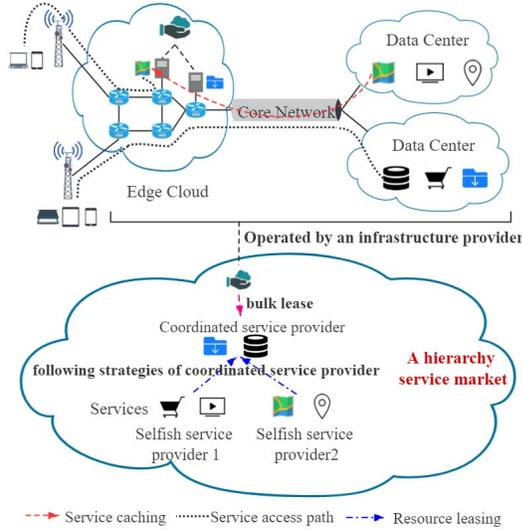
Fig. 1. An example of the two-tiered cloud network.
