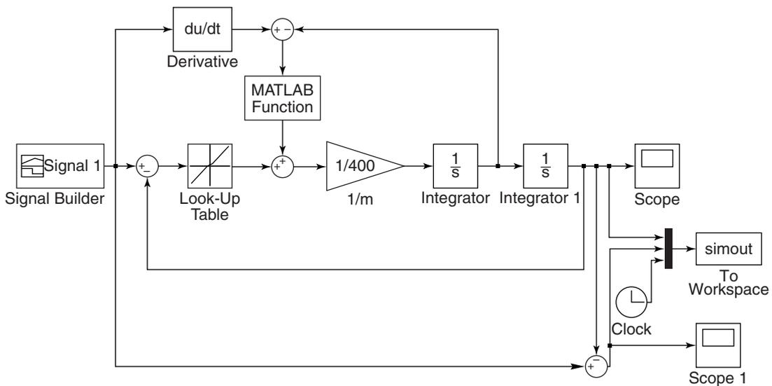
Figure 10.9-6 Simulink model of a vehicle suspension system.
