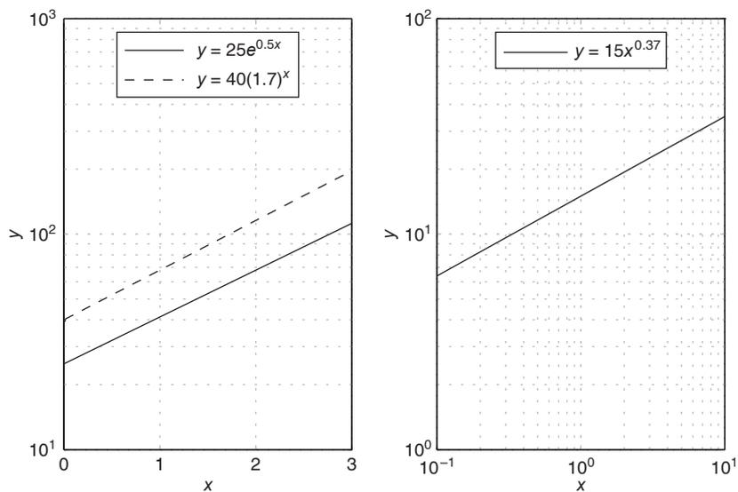
**Figure 5.2-6** Two examples of exponential functions plotted with the `semilogy` function (the left-hand plot), and an example of a power function plotted with the `loglog` function (right-hand) plot.
