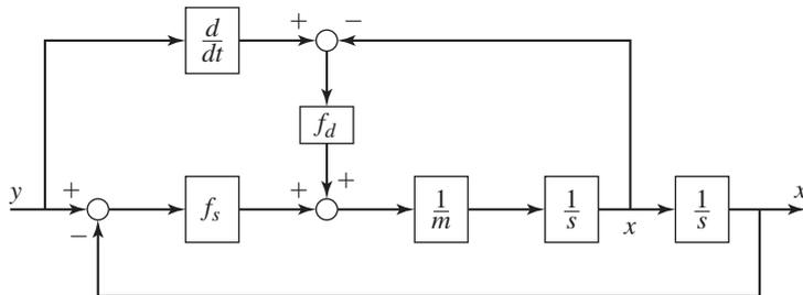
Figure 10.9-5 Simulation diagram of a vehicle suspension model.
