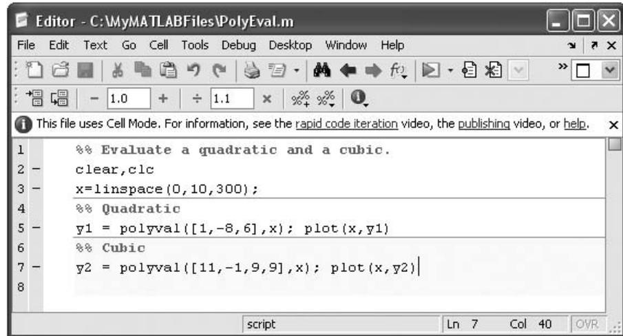
Figure 4.8–2 The cell mode of the Editor/Debugger.
