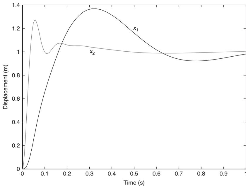
**Figure 10.3–3** Unit-step response of the two-mass suspension model.
