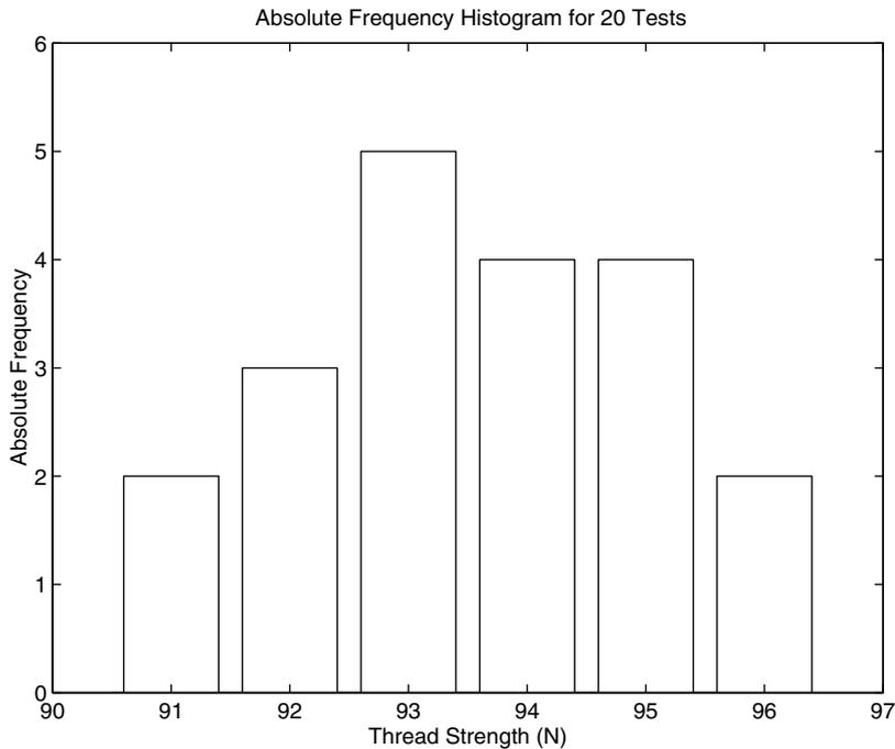
Figure 7.1-1 Histograms for 20 tests of thread strength.
