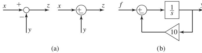
**Figure 10.1-2** (a) The summer element. (b) Simulation diagram for  $\dot{y} = f(t) - 10y$ .
