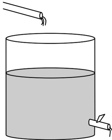
**Figure 6.1–4** An experiment to verify Torricelli's principle.
