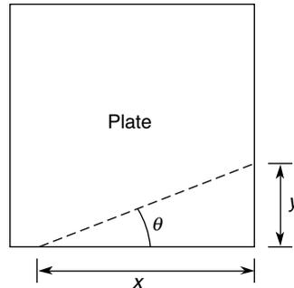
**Figure 7.3-1** Dimensions of a triangular cut.
