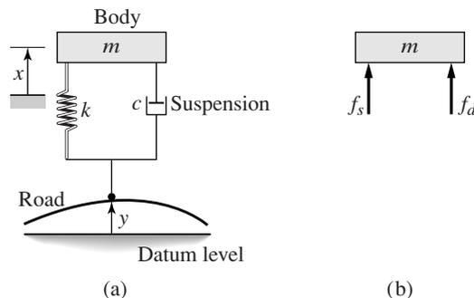
Figure 10.9–1 Single-mass model of a vehicle suspension.
