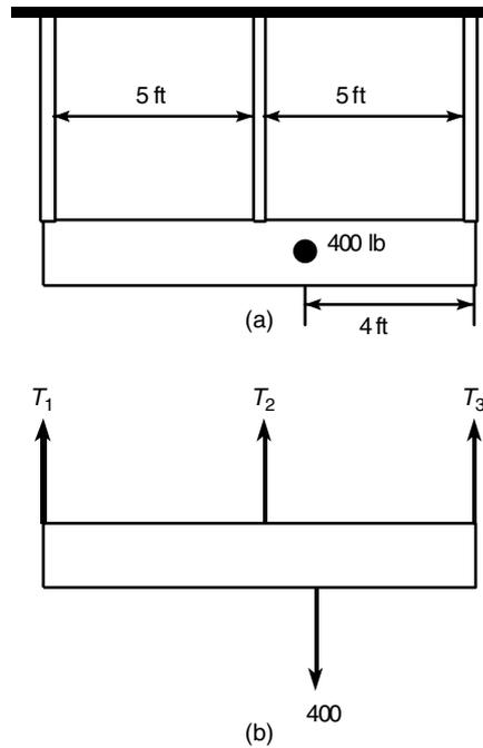
Figure 8.3-1 A light fixture and its free-body diagram.
