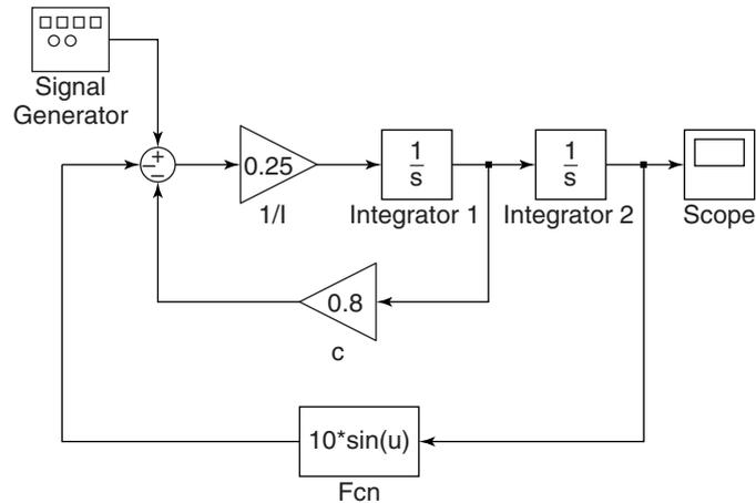
Figure 10.6–2 Simulink model of nonlinear pendulum dynamics.
