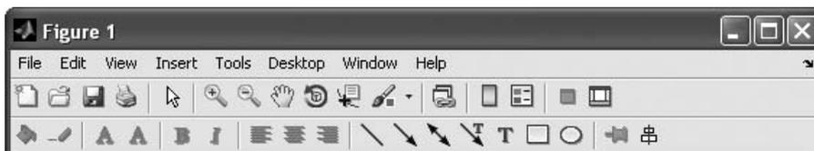
Figure 5.3–2 The Figure and Plot Edit toolbars displayed.
