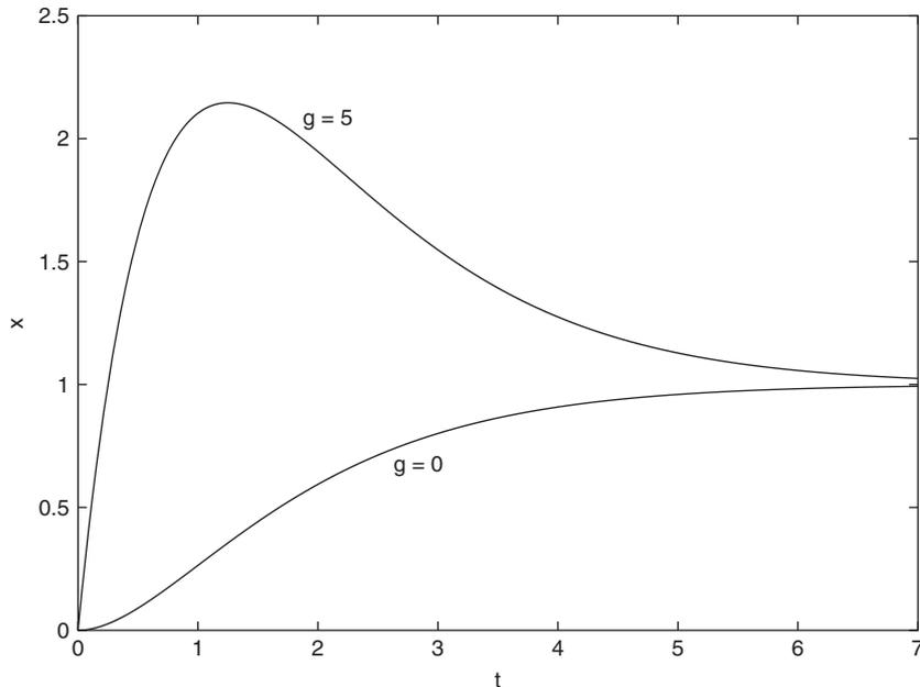
**Figure 11.7-2** The step response of the model  $\ddot{x} + 2\dot{x} + x = u + gu$  for  $g = 0$  and  $g = 5$ .
