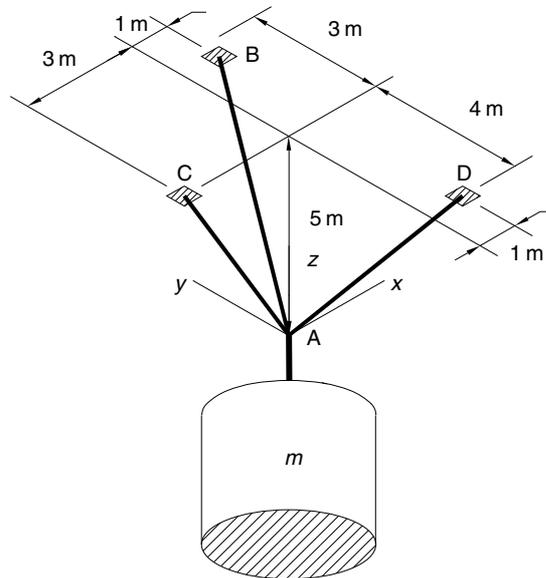
Figure 8.2–1 A mass suspended by three cables.
