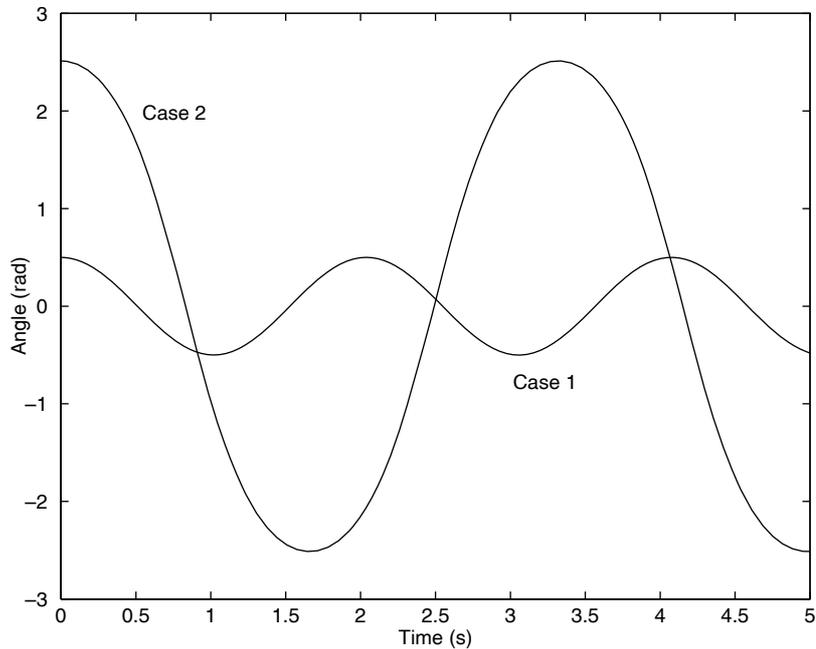
**Figure 9.4-2** The pendulum angle as a function of time for two starting positions.
