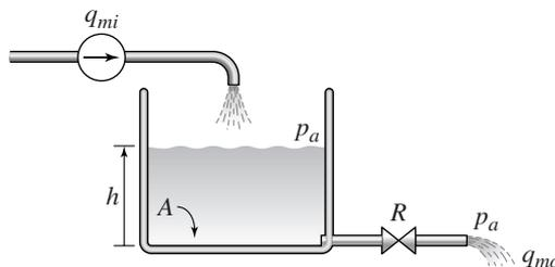
**Figure 10.7–1** A hydraulic system with a flow source.
