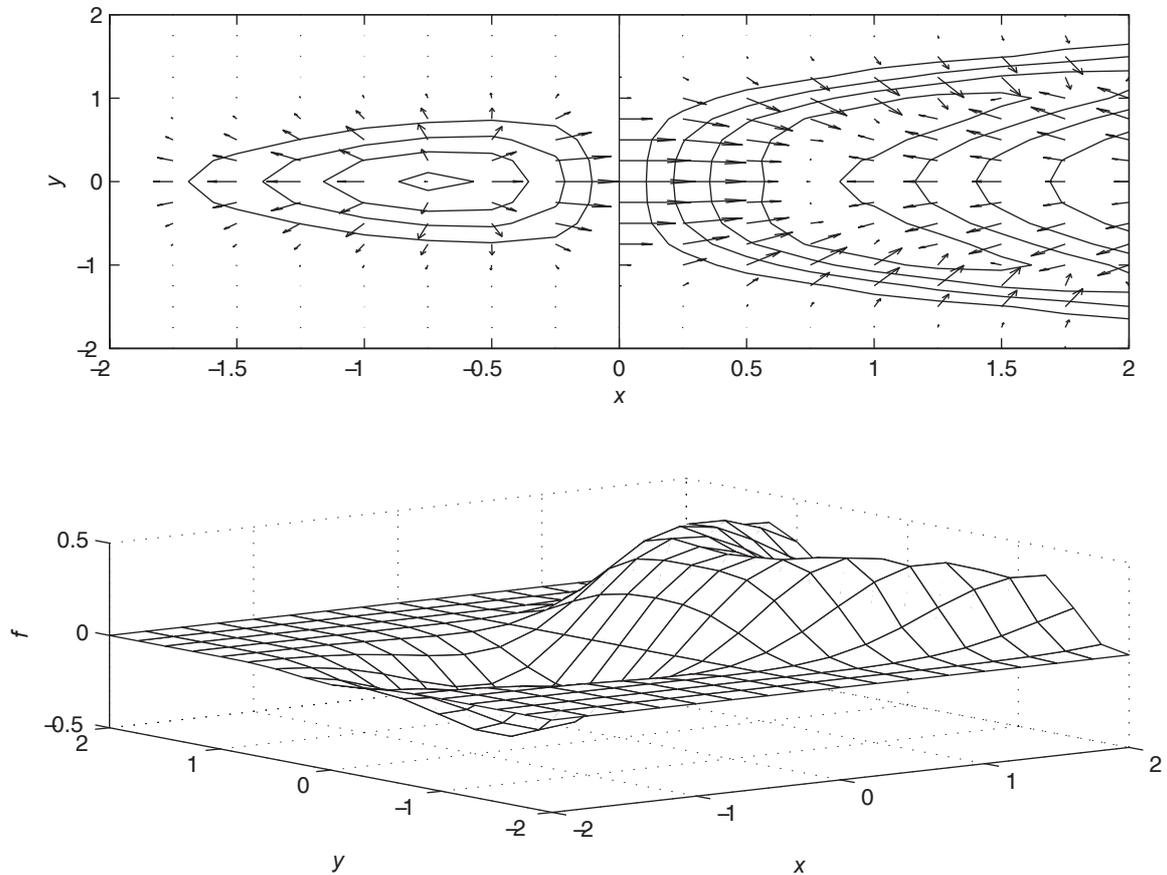
**Figure 9.2-2** Gradient, contour, and surface plots of the function  $f(x, y) = xe^{-(x^2+y^2)} + y^2$ .
