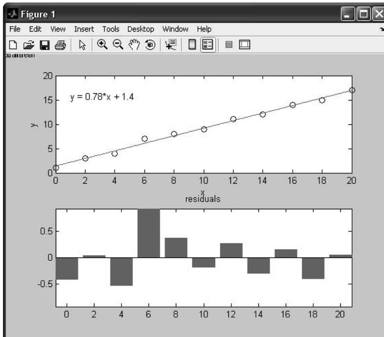
Figure 6.3–2 A figure produced by the Basic Fitting interface.
