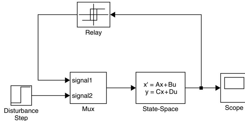
Figure 10.4–9 Simulink model of a relay-controlled motor.
