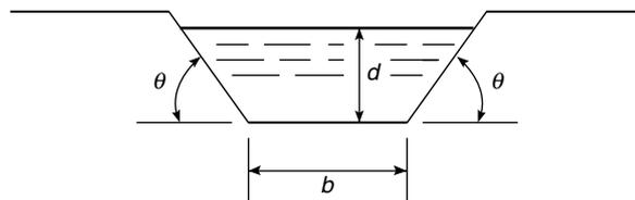
Figure 3.2–3 Cross section of an irrigation channel.
