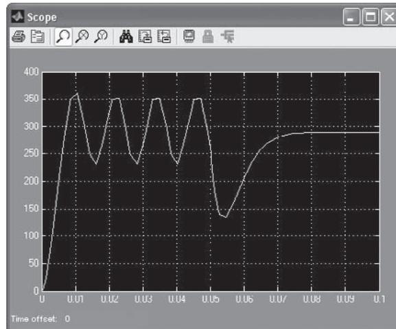
**Figure 10.4–10** Scope display of the speed response of a relay-controlled motor.
