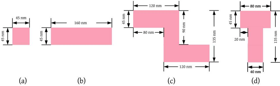
Fig. 11. Restricted set of patterns for black-box attack (shape dimensions shown). The (a) square, (b) rectangle, (c) zigzag, and (d) Tee shapes are drawn from the existing layout dataset.
