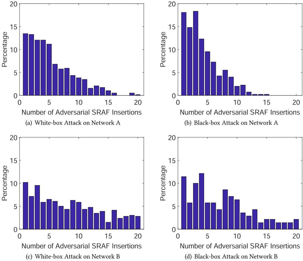
Fig. 7. Histograms of percentages of different number of adversarial SRAF insertions by white-box attack on Networks A (a) and B (c). Histograms of percentages of different number of adversarial SRAF insertions by black-box attack on Networks A (b) and B (d).
