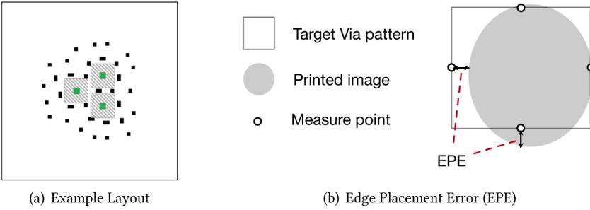
Fig. 3. (a) Example of a layout with vias (in green), SRAFs (in black), and the forbidden areas (striped region). (b) Illustration of edge placement error (EPE). Each target via pattern has four measure points (one at the center of each edge). The EPE is the perpendicular displacement from the measure point to the corresponding printed image (contour).
