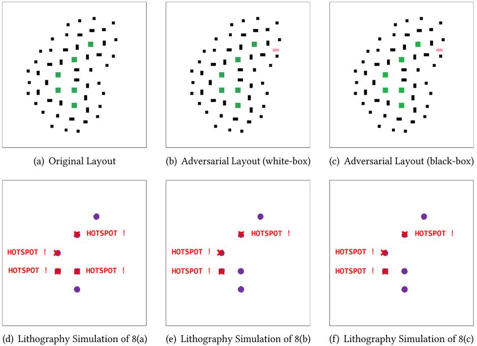
Fig. 8. White-box and black-box attack outputs—Example 1. These examples feature a single inserted SRAF. In the layout images (a–c), the vias are colored green, the original SRAFs are black, and the adversarial SRAFs are red. In the lithography simulation outputs, the vias are shown in purple and hotspots are marked with a cross and labelled with “HOTSPOT!”
