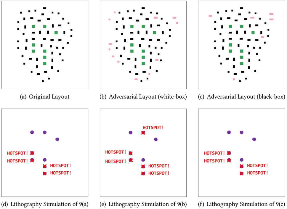
Fig. 9. White-box and black-box attack outputs—Example 2. These examples feature multiple inserted SRAFs. In the layout images (a–c), the vias are colored green, the original SRAFs are black, and the adversarial SRAFs are red. In the lithography simulation outputs, the vias are shown in purple and hotspots are marked with a cross and labelled with “HOTSPOT!”
