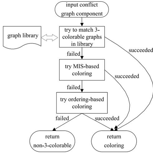
Fig. 11. Flow of 3-colorability checking.
