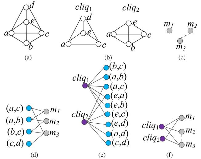
Fig. 12. Illustration for K4-based move selection in CRMA<sub>3</sub>. Dashed line is incompatible edge between moves. (a) Conflict graph  $G$ . (b) Identified K4s  $cliq_1$  and  $cliq_2$ . (c) Move constraint graph. (d) Bipartite graph  $B_1$  between  $\mathcal{C}_f$  and  $\mathcal{M}$ . (e) Bipartite graph  $B_2$  between  $\mathcal{C}_q$  and  $\mathcal{C}_f$ . (f) Integrated graph model. Note that (c) and (d) are assumed the same as those in Fig. 6 for simplicity.
