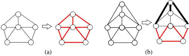
Fig. 14. Illustration for critical edges. Highlighted critical edges in a graph (a) in the library and (b) out of the library.
