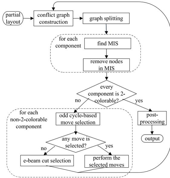
Fig. 9. Flow of the baseline method for CRMA<sub>3</sub> that reduces CRMA<sub>3</sub> to CRMA<sub>2</sub>.
