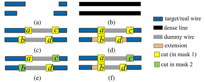
Fig. 1. (a) 1-D target layout. (b) Dense lines. (c) Cuts and dummy wires. (d) Cuts are redistributed. (e) Cuts are assigned to different masks. (f) Incorporating cut redistribution with cut mask assignment.
