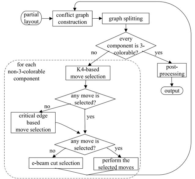
Fig. 10. Flow of our method K4solver for CRMA<sub>3</sub> that solves CRMA<sub>3</sub> directly.
