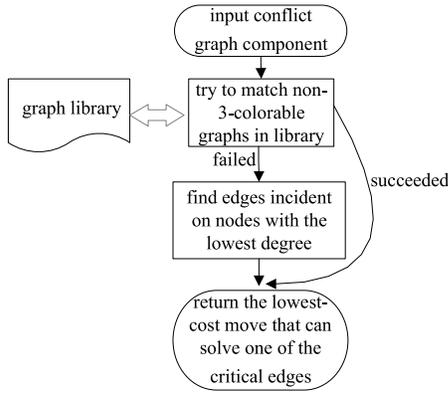
Fig. 13. Flow of critical edge-based move selection.
