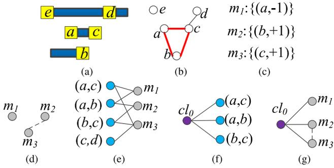
Fig. 6. Illustration for odd cycle-based move selection in CRMA<sub>2</sub>. Dashed line is incompatible edge between moves.  $cl_0$  is the cycle of  $a$ ,  $b$ , and  $c$ . (a) Cuts. (b) Conflict graph  $G$ , and the odd cycle in its cycle basis is highlighted. (c) Moves. (d) Move constraint graph. (e) Bipartite graph  $B_1$  between  $C_f$  and  $\mathcal{M}$ . (f) Bipartite graph  $B_2$  between  $C_l$  and  $C_f$ . (g) Integrated graph model.
