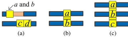
Fig. 2. Different types of merging. (a) Merging on the same track.  $a$  is merged with  $b$ .  $c$  is merged with  $d$ . (b) Cuts  $a$  and  $b$  on adjacent tracks are merged. (c) Cuts  $a$  and  $c$  on nonadjacent tracks are merged. In such case,  $a$ ,  $b$ , and  $c$  should be vertically aligned.
