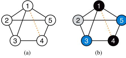
Fig. 9. Simple example of SDP. (a) Input DG component. (b) Color assignment result with 0 conflict and 0 stitch.
