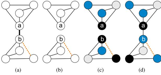
Fig. 12. Bridge edge detection and removal. (a) Initial DG. (b) After bridge edge detection, remove edge  $e_{ab}$ . (c) In two components, we carry out layout decomposition. (d) Rotate colors in the lower component to add bridge.
