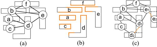
Fig. 2. Layout graph construction and DG construction. (a) Layout graph for given input, where all edges are conflict edges. (b) Vertex projection. (c) Corresponding DG, where dash edges are stitch edges.
