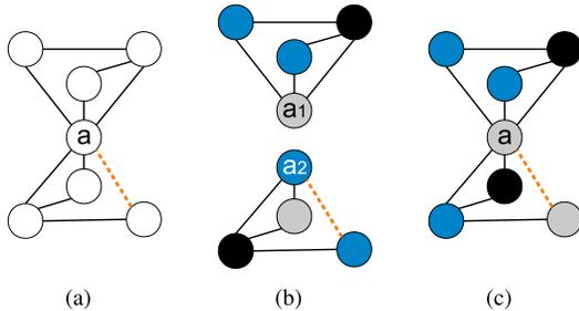
Fig. 13. Bridge vertex detection and duplication. (a) Initial DG. (b) After bridge vertex detection, duplicate vertex  $a$ . (c) Rotate the colors in lower sub-graph to merge vertices  $a_1$  and  $a_2$ .
