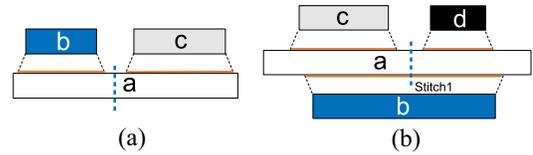
Fig. 5. Examples of (a) redundant stitch and (b) lost stitch.
