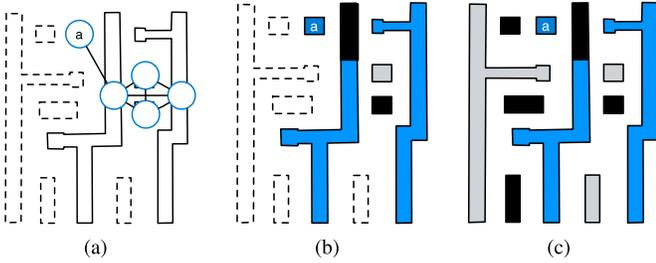
Fig. 15. Example of post-refinement. (a) Extend LG to include  $a$ . (b) Stitch generation and color assignment on the new graph. (c) No additional conflict at final solution.
