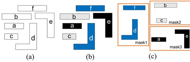
Fig. 1. Example of TPLD. (a) Input layout. (b) Features with different colors mean that they are assigned into different masks. (c) Features on each mask.
