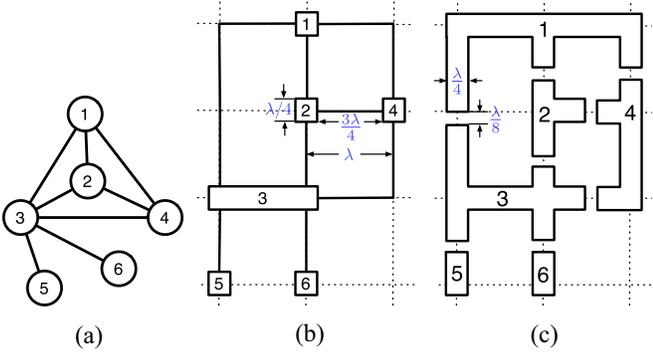
Fig. 3. Reducing PG3C to TPLD. (a) Instance of PG3C. (b) Transferred orthogonal drawing. (c) Corresponding TPLD instance.
