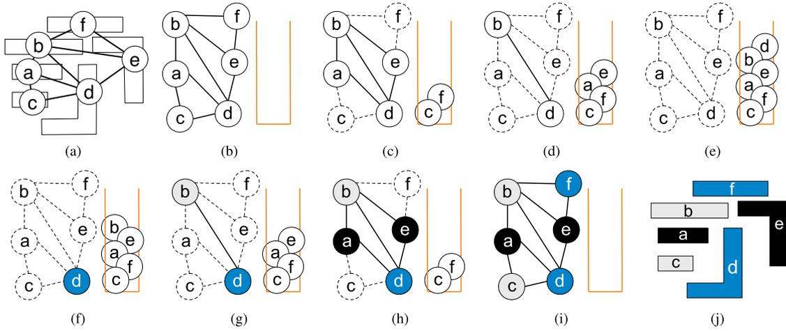
Fig. 11. Example of IVR, where the TPLD problem can be solved in linear time. (a) LG. (b)–(e) Iteratively remove and push in vertices with degree less than three. (f)–(i) After color assignment for the remanent vertices, iteratively pop-up and recover vertices, and assign any legal color. (j) TPLD can be finished after the iterative vertex recover.
