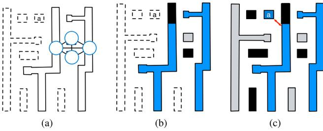
Fig. 14. IVR may introduce additional conflicts. (a) LG after IVR. (b) Stitch generation and color assignment on the graph. (c) After adding back the simplified vertices, one additional conflict is introduced to vertex  $a$ .
