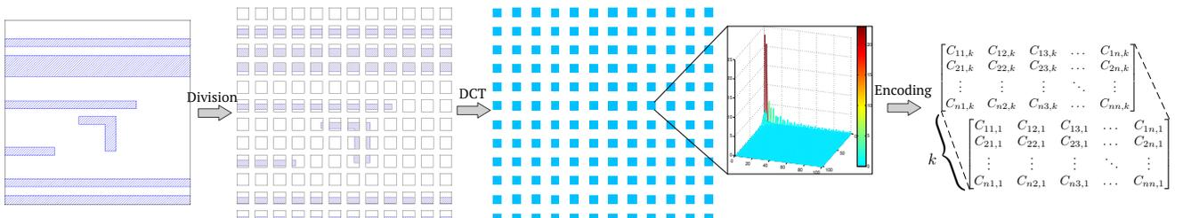
**Figure 1:** Feature Tensor Generation Example ( $n = 12$ ). The original clip ( $1200 \times 1200 \text{ nm}^2$ ) is divided into  $12 \times 12$  blocks and each block is converted to  $100 \times 100$  image representing  $100 \times 100 \text{ nm}^2$  sub region of the original clip. Feature tensor is then obtained by encoding DCT coefficients of each block.
