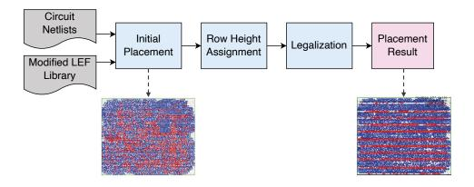
Traditional flow causes significant disruptions in the initial placement results, resulting in inferior wirelength.
