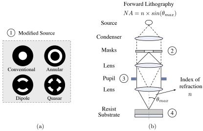
Figure 1: (a) Different representations of illuminator source, conventional source, annular source, dipole source, ans quasar source. (b) Core components of forward lithography process.
