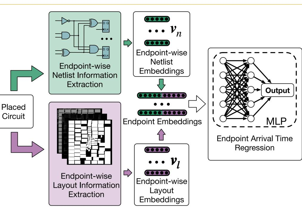
Figure 2. Overview of our pre-routing timing prediction framework, which first generates endpoint-wise embedding and then conducts sign-off global timing prediction.
