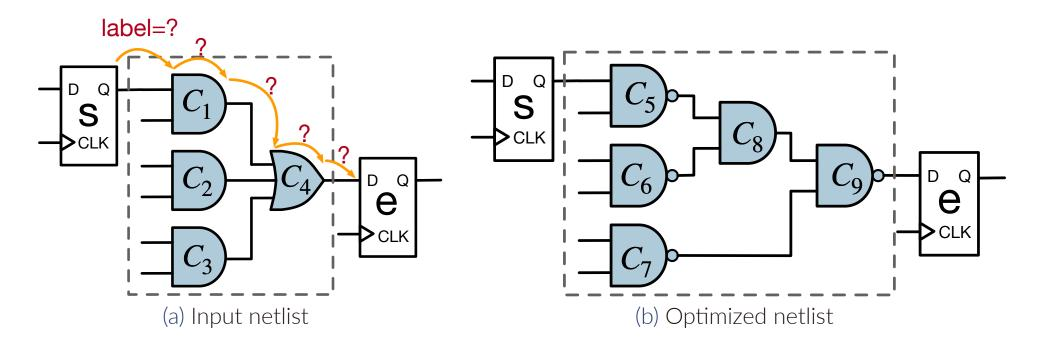
Figure 1. Example of circuit reconstruction after timing optimization
