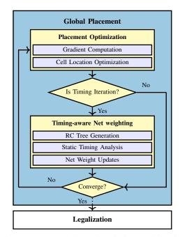
Fig. 1 Our overall flow with timing optimization.
