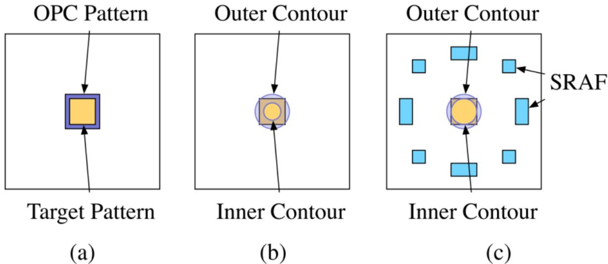
**Problem definition:** Given a design image  $\vec{w}$ , the objective of mask optimization is generating the corresponding mask  $\vec{x}$  such that remaining patterns  $\vec{y}$  after lithography process is as close as  $\vec{w}$  or, in other words, minimizing PV Band and squared  $L_2$  error of lithography images.
