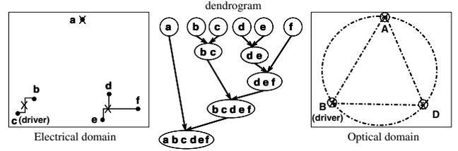
Figure 4: A brief illustration of netlist pre-processing
