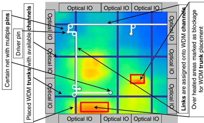
Figure 5: Our WDM based global routing scenario
