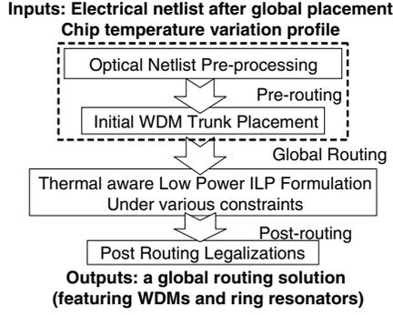
Figure 3: An overview of our proposed CAD flow
