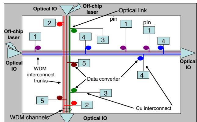
Figure 1: High routing capacity interconnect using WDM
