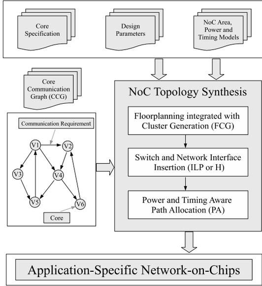
Fig. 1. NoC Design Approach Overall
