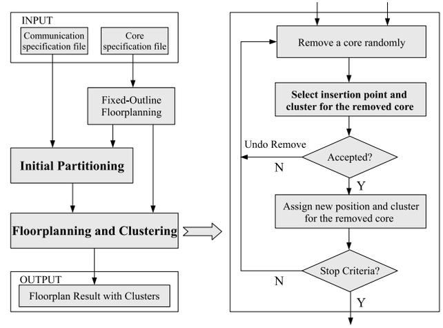
Fig. 2. Floorplanning integrated with Cluster Generation (FCG)
